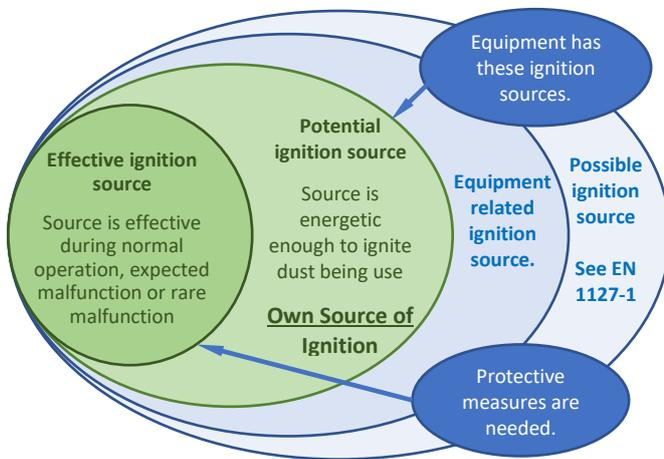
The minimum ignition energy (MIE) of a dust cloud has a significant impact on whether a source of ignition will be an effective source of ignition. EN ISO 80079-36 includes the hierarchy of sources of ignition illustrated in the diagram on the left. Although this relates to sources of ignition caused by equipment, it is equally relevant to sources of ignition created by a process.
