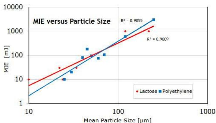
To find the actual MIE a much larger number of tests are required varying the test energy in much smaller steps and carrying out the test over a wide range of sample sizes. However, since the MIE is also a function of particle size and moisture content as shown in the graphs to the left and below, it is unlikely that the additional cost of this extra testing will be worthwhile for most industrial plants.
